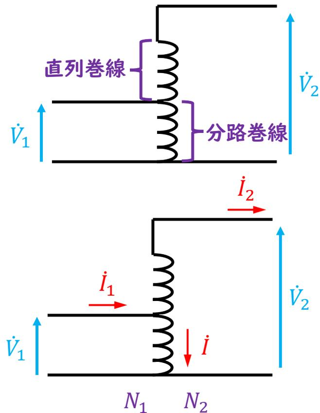
$$\begin{aligned} \text{自己容量} &= \text{直列巻線の容量} = \text{分路巻線の容量} \\ &= (V_2 - V_1)I_2 = V_1(I_1 - I_2) \end{aligned}$$
