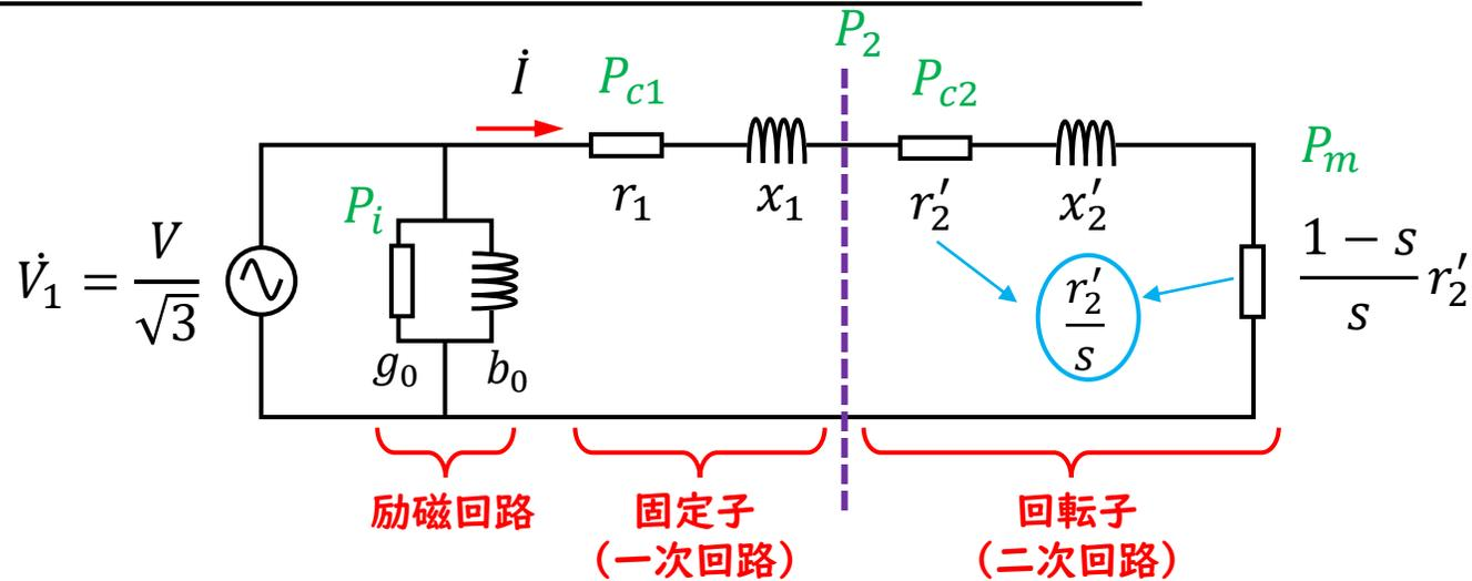
$$I = \frac{V_1}{\sqrt{\left(r_1 + \frac{r'_2}{s}\right)^2 + (x_1 + x'_2)^2}}$$
