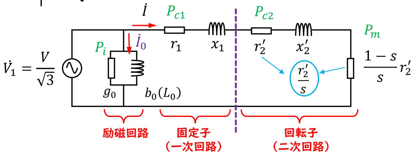
$$T = \frac{P_2}{\omega_s} = \frac{1}{\omega_s} \left( 3 \frac{r_2'}{s} I^2 \right) = \frac{3}{2\pi \frac{1}{60} \frac{120}{p}} \frac{\frac{r_2'}{s} \left( \frac{V_1}{f} \right)^2}{\left( r_1 + \frac{r_2'}{s} \right)^2 + (x_1 + x_2')^2}$$
